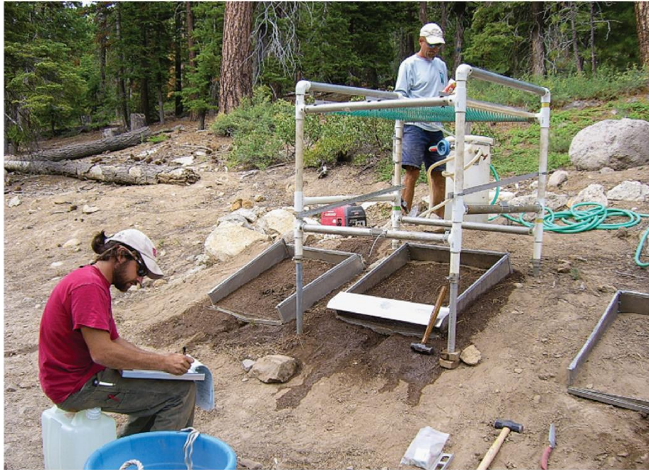
Rainfall simulators are used by researchers to measure erosion and the loading of sediments into streams. UC Davis hydrology professor Mark Grismer (right) and GIS specialist Lee Perlow collect data using a simulator installed on a bare soil slope above Kings Beach, Lake Tahoe.
